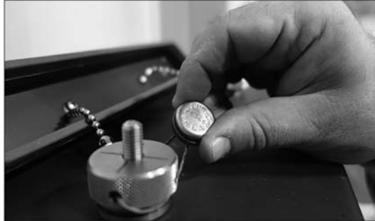
Figure 3: An Inspector Replaces a Seal
