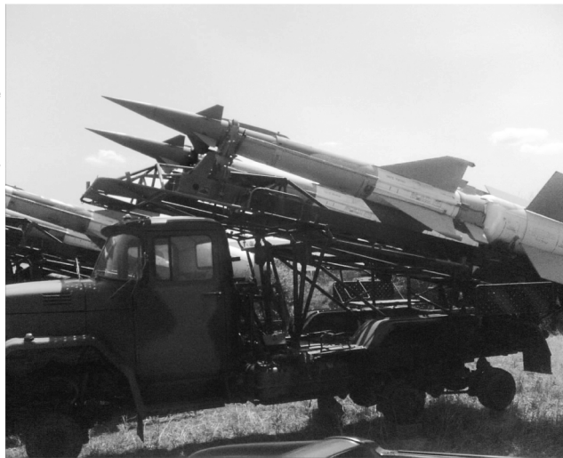
A Georgian surface-to-air missile system with an operational range of approximately 15 miles. The missiles are about 18 feet long and travel at speeds exceeding Mach 3.
